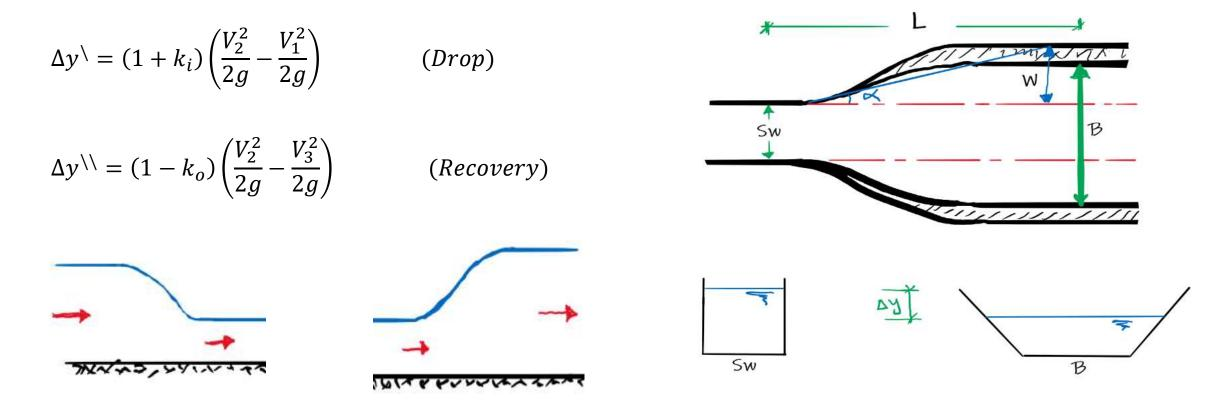
♦ Calculate the water surface profile, equation as a parabola function  $Y = CX^2$ .
