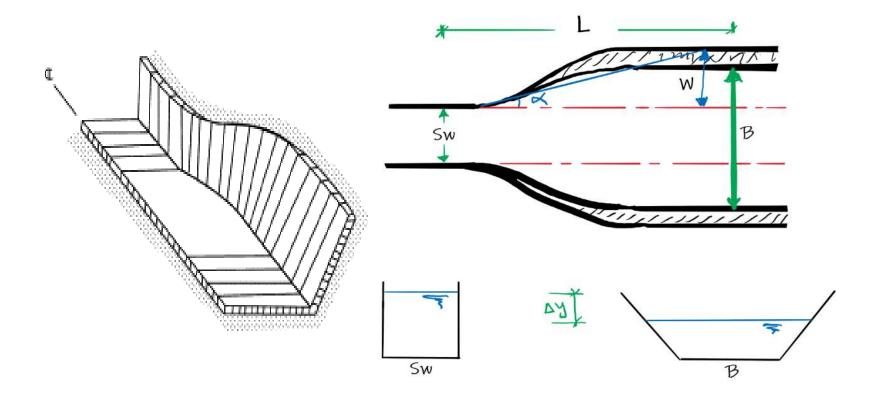
• Length of the transition. To determine the length of the transition, a straight line joining the flow line (on the wall) at the two ends of the transition should make an angle ( $\theta$ ) with the longitudinal alignment.
