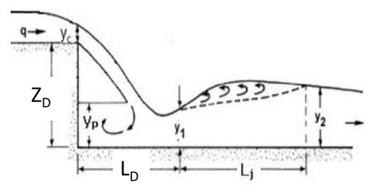
**Example**: Design a vertical drop structure in a lined canal carrying a normal discharge of  $5m^3$ /sec to lower the water from the U/S to D/S by 2m. The canal cross section in the reach's U/S and D/S of the structure are same and given below: -
