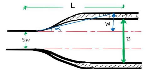
$$\Delta y^{\backslash \backslash} = (1 - k_o) \left( \frac{V_2^2}{2g} - \frac{V_3^2}{2g} \right)$$
